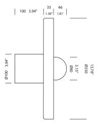
Installation note: Comes with a 4" backplate that mounts to a standard junction box
