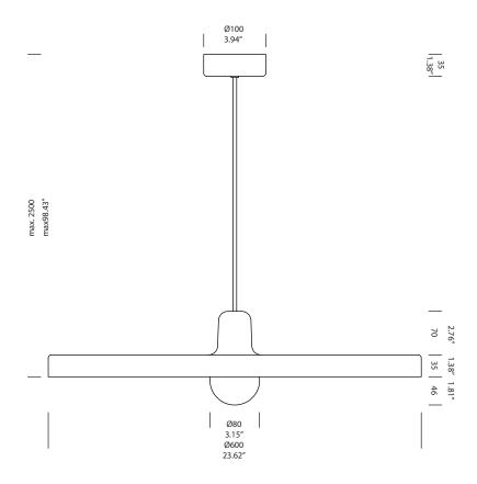
Installation note: Comes with a 4" backplate that mounts to a standard junction box
