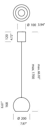
Installation note: Comes with a 4" backplate that mounts to a standard junction box
