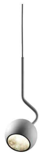
SPIN is an adjustable pendant luminaire interpreting the classic sphere – with a special feature. Thanks to the excentric mounting point the light direction can be adapted most easily. With SPIN changing the lighting mood is just one turn away. Even being familiar in appearance the inner life is equipped with up to date LED technology. A simple yet smart mounting unit simplifies changing the reflector which is available with different angles of radiation.
